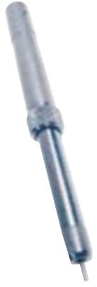
Tang break off tools are available in hand, semi automatic spring type and pneumatic. The spring loaded and pneumatic tang break tools are recommended for removal of tangs in production applications. For large diameter fine thread inserts, e.g. M18-1.5 and above, 3/4-16 and above, the use of long nose pliers is an alternative method to break the tang.
