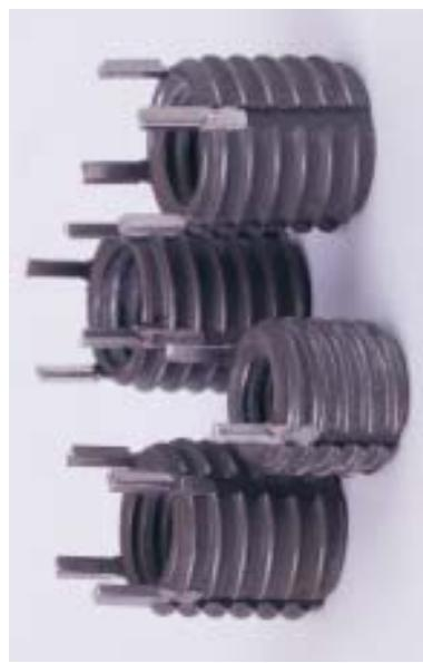
Keyserts from Alcoa Fastening Systems provide an easy-to-install thread assembly to replace damaged, stripped or worn threads in a wide range of materials including castings, forgings and mechanical components (except cast iron or sintered materials).
